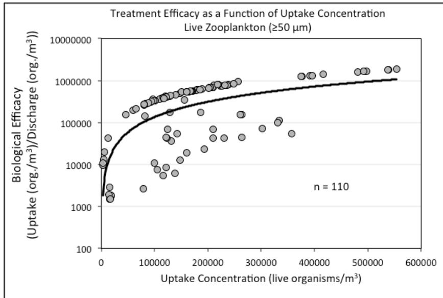
relation to the final discharge concentration of living organisms after ballast treatment; e.g., a simple comparison of 'what goes in vs. what goes out' (Figure). The reduction value (uptake live concentration ÷ discharge live concentration; y axis of Figure) as a function of incoming challenge concentration (x axis) ranged from 1,000x to over 1,000,000x; more than half of the comparisons fell in the range 100,000x to
